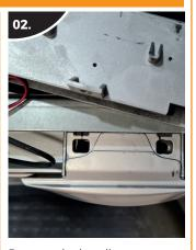
Remove the handle mechanism from the door, there are two screws accessible from the top to do this.
