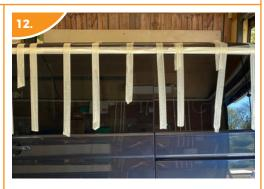
Once you are happy with the glass positioning and it's all taped up, remove protective masking (but not tape holding the glass in place), vacuum out the metal / dust in the rear of the vehicle and have a cup a tea.
