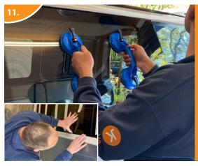
Before you lift the glass up, put 2x 400mm lengths of 50mm wide masking tape loosely
