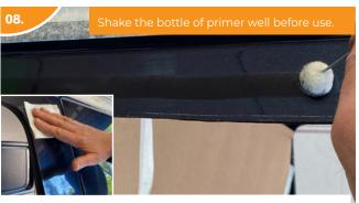
Clean the panel work with the alcohol wipes. Now apply the primer in a line, remembering the same will be done on the glass and between the two lines of primer will sit the bonding mastic.
