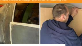
Making sure the vehicle is clean, mask the vehicle up fully. You'll be amazed how far sparks can travel and the may burn into your paint and damage interiors very easily.
