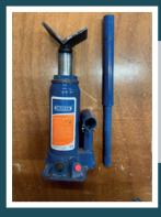
"Depending on the car and state of the jacking points, I either carry an original jack, or I made up my own version of a bottle jack with some angle iron properly welded to the top."
