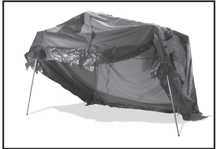
2. Lay awning material over the top of the frame
