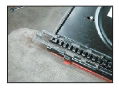
7. The last job to do is to put your seat back into its runners. Before you do this though make sure you have removed any swarf from the runners. Rotate the seat base back into its forward position until it locks into place then push the seat onto the runners until it clicks past the stop.
