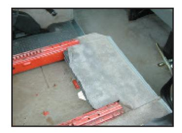
4. Position the swivel seat base over the vehicle runners. You can see that only four of the holes line up, there is a larger diagram on the last page giving you dimensions to drill out the two extra holes. Please note that also two of the exisiting holes in the runners need to be drilled out to 8.5mm, again full details are on the last page.
