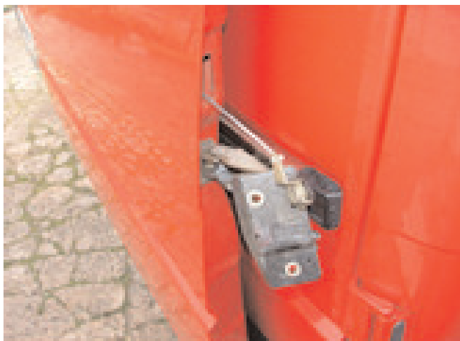
STEP 3: Pull the latch assembly out with the rod. Once the rod has cleared the inner skin, replace it so that the rod passes to the inside of the inner skin. Refit the rear latch.
