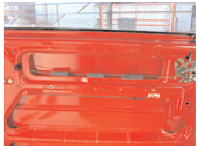
STEP 4: Refit the rod to the front latch and reprofile so it clears the panel work. Open and shut the door several times to ensure the door closes correctly, if it does not catch every time, adjust the rod until correct.
