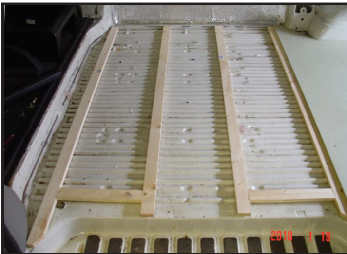
B. Bond wooden battens to the floor.
