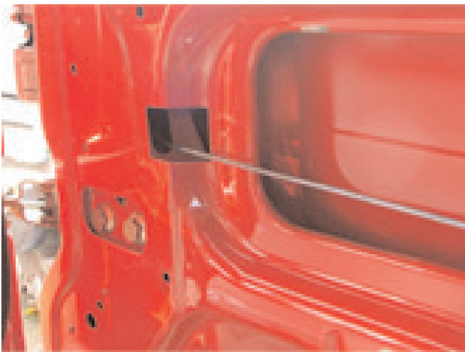
STEP 1: Remove the door rod from the front latch, this is
