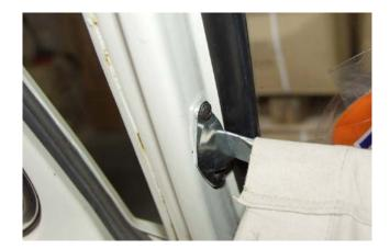
5. Feed the rail through the tube within the canvas, making sure the rails face inwards. Connect the front rail into both brackets.
