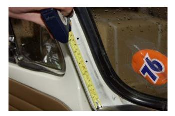
2. Now measure from the seam (not the window rubber) 10mm and draw a line creating a cross. This will be the lower hole for the bracket. Drill through the cross.
