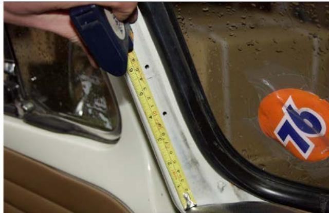
2. Now measure from the seam (not the window rubber) 10mm and draw a line creating a cross. This will be the lower hole for the bracket. Drill through the cross.
