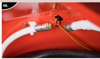
In some cases, you may struggle to find suitable places to attach the hose to and you can use self-adhesive cable tie mounts that are available cheaply from places like Screwfix, Toolstation and B&Q etc.
