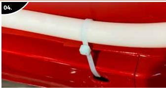
Think about where a fire is most likely to happen and install as much of the hose over these areas as possible. In our experience, this is where the fuel pump and carburettor(s) are. Find suitable points above these areas to cable tie the hose to.
