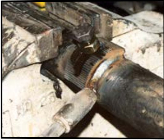
9. Weld the adjuster
