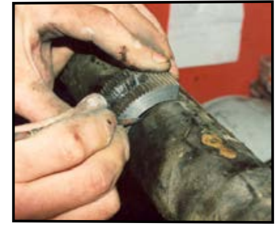
6. Use the adjuster to scribe the beam
