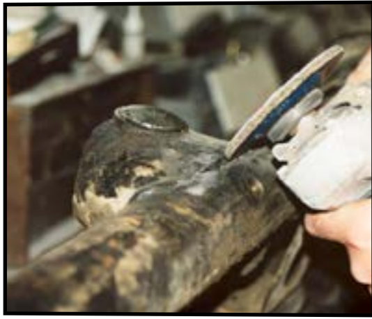
1. Carefully cut off knuckle
