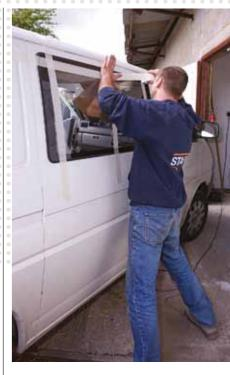
15 Use plenty of masking tape to hold the new window in place. You can't drive the vehicle for at least 24 hours whilst the adhesive sets. It goes without saying that it's a good idea to have somewhere out of the elements to store the Bus for this period of time
