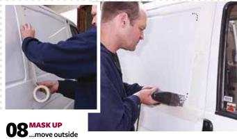
now and you'll see your pilot holes in the corners of the panel to be removed. Run some masking tape to protect the paintwork and then grab your jigsaw. You can make life a little easier for your jigsaw blade by enlarging the holes with a fatter drill bit but it isn't strictly necessary. Now simply join the dots, but take it easy and let the blade do the work
