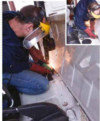
06 BRUTE A cold chisel and hammer will come in handy, too. The bulkhead is a tight fit and these 'precision tools' can be used to break any remnants of the spot welds. A good shove from behind and our bulkhead came free no problem. If yours is stubborn, go round the edges and check again for hang ups
