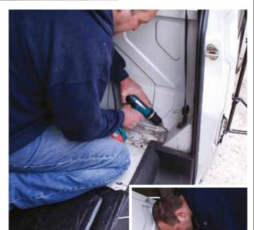
**Q4** DRILL With the interior stripped out, it's time to break out the power tools. Type 2s are simple creatures so you can easily see where they're spot welded together. Work your way along the bulkhead and drill out all of the spot welds. Having a couple of spare drill bits on hand is a good idea as breakages can slow you down. You can use a centre punch on the spot welds to guide a normal drill bit, but it's easier and quicker to buy a proper spot weld drill bit
