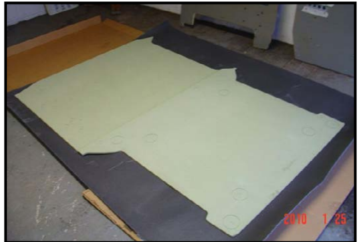
E. Lay the floor boards on the flooring in reverse.
